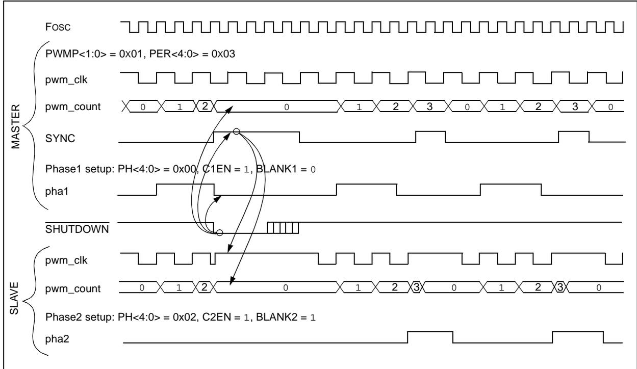
**FIGURE 13-3: TWO-PHASE PWM START-UP TIMING**
