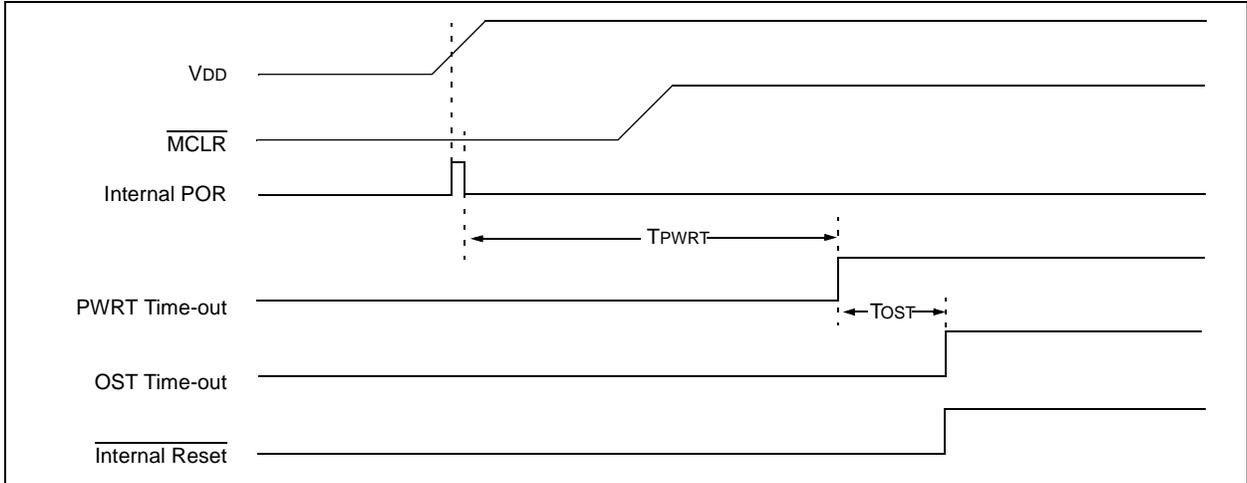
**FIGURE 15-5: TIME-OUT SEQUENCE ON POWER-UP (DELAYED  $\overline{\text{MCLR}}$ ): CASE 2**
