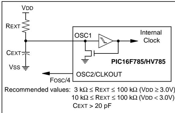
In RCIO mode, the RC circuit is connected to the OSC1 pin. The OSC2 pin becomes an additional general purpose I/O pin. The I/O pin becomes bit 4 of PORTA (RA4). Figure 3-6 shows the RCIO mode connections.
