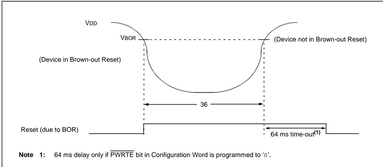
**TABLE 19-4: RESET, WATCHDOG TIMER, OSCILLATOR START-UP TIMER, POWER-UP TIMER AND BROWN-OUT RESET REQUIREMENTS**
