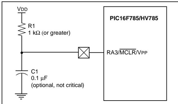
An internal  $\overline{\text{MCLR}}$  option is enabled by clearing the MCLRE bit in the Configuration Word. When cleared,  $\overline{\text{MCLR}}$  is internally tied to VDD and an internal Weak Pull-up is enabled for the MCLR pin. The VPP function of the RA3/MCLR/VPP pin is not affected by selecting the internal  $\overline{\text{MCLR}}$  option.
