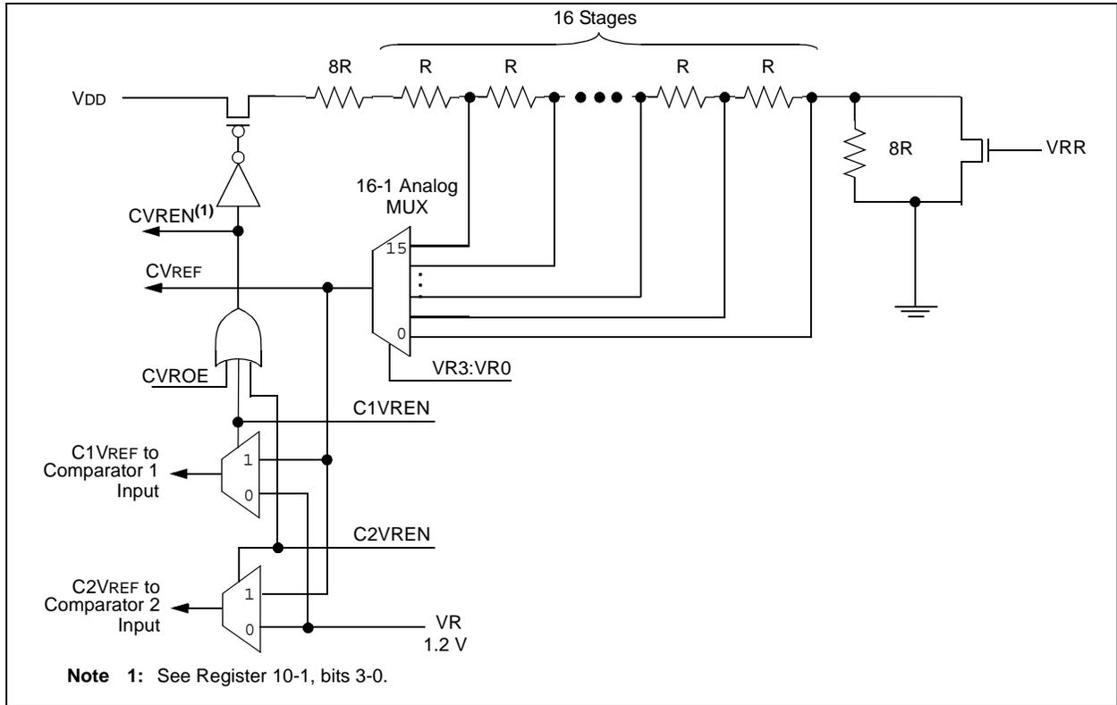
**REGISTER 10-1: VRCON: VOLTAGE REFERENCE CONTROL REGISTER (ADDRESS: 99h)**
