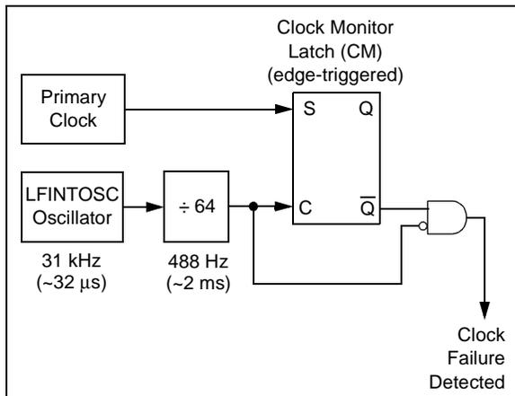
On the rising edge of the sample clock, the monitoring latch (CM = 0) will be cleared. On a falling edge of the primary system clock, the monitoring latch will be set (CM = 1). In the event that a falling edge of the sample clock occurs, and the monitoring latch is not set, a clock failure has been detected. The assigned internal oscillator is enabled when FSCM is enabled as reflected by the IRCF bits.
