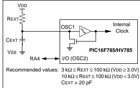
The RC oscillator frequency is a function of the supply voltage, the resistor (REXT) and capacitor (CEXT) values and the operating temperature. In addition to this, the oscillator frequency will vary from unit-to-unit due to normal threshold voltage. Furthermore, the difference in lead frame capacitance between package types will also affect the oscillation frequency or low CEXT values. The user also needs to take into account variation due to tolerance of external RC components used.
