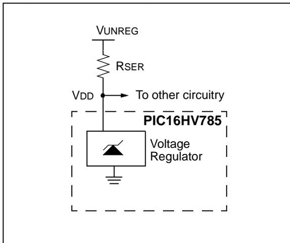
An external current limiting resistor, R<sub>SER</sub>, located between the unregulated supply, V<sub>UNREG</sub>, and the VDD pin, drops the difference in voltage between V<sub>UNREG</sub> and VDD. R<sub>SER</sub> must be between R<sub>MAX</sub> and R<sub>MIN</sub> as defined by Equation 16-1.
